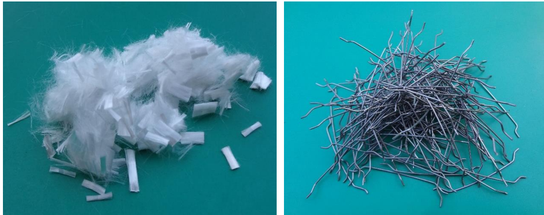
Figure 4. Fibers used in the study: (a) steel fibers and (b) polypropylene fibers.
