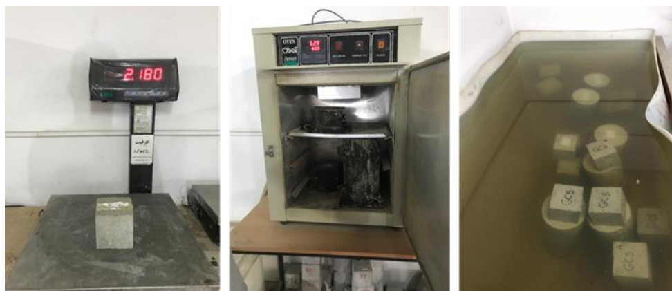
Figure 7. Weighing and drying of geopolymer samples
